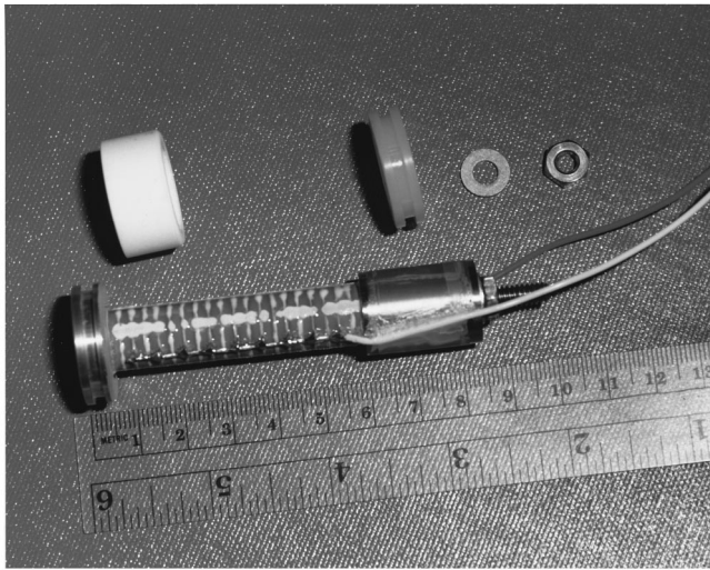
FIG. 5. Photograph of assembled driver, consisting of ring stack, head and tail masses, and tie rod. Also shown as separate parts are (from left) the syntactic foam isolator, the nylon tail support, and the washer and nut that secure the tail support.
